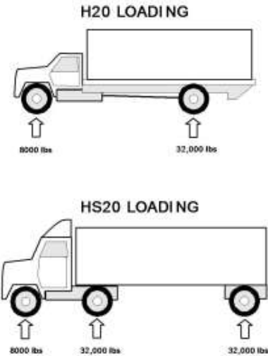
Figure 1. H-20 and HS-20 Loading
